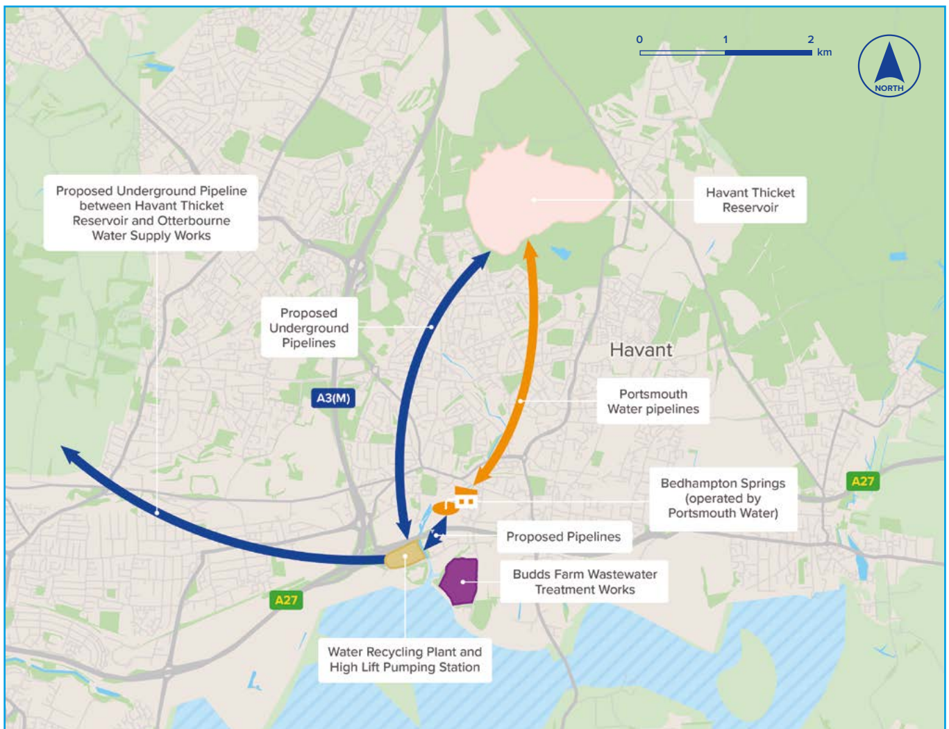
Graphic 3-4 Proposed Pipelines between the proposed Water Recycling Plant and Havant Thicket Reservoir
