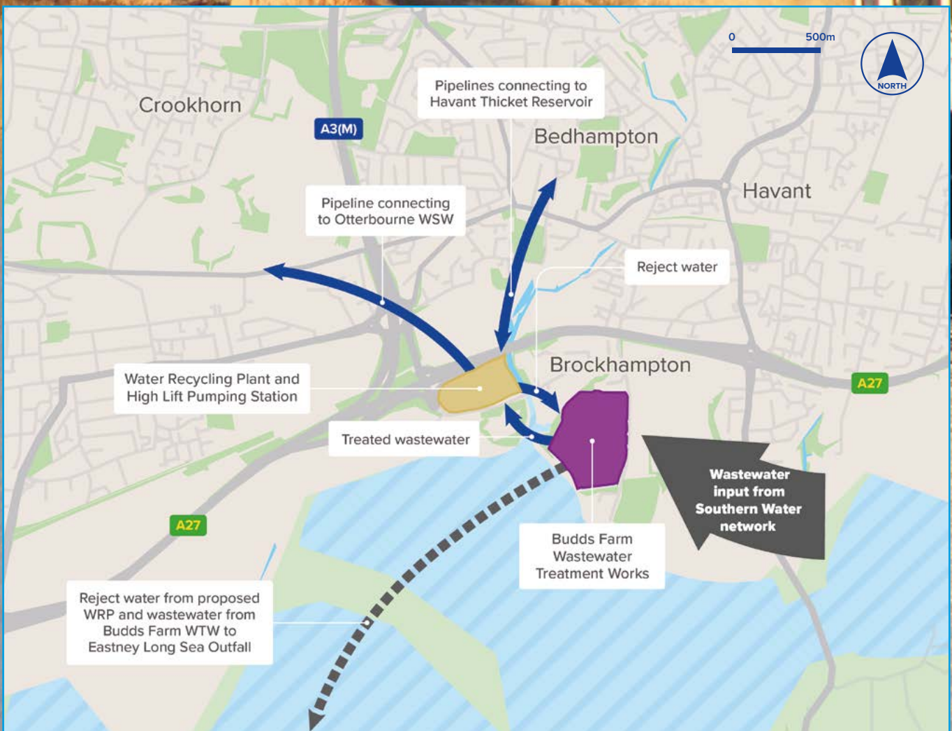
Graphic 3-3 Proposed Underground Pipelines between Budds Farm Wastewater Treatment Works and the proposed Water Recycling Plant
