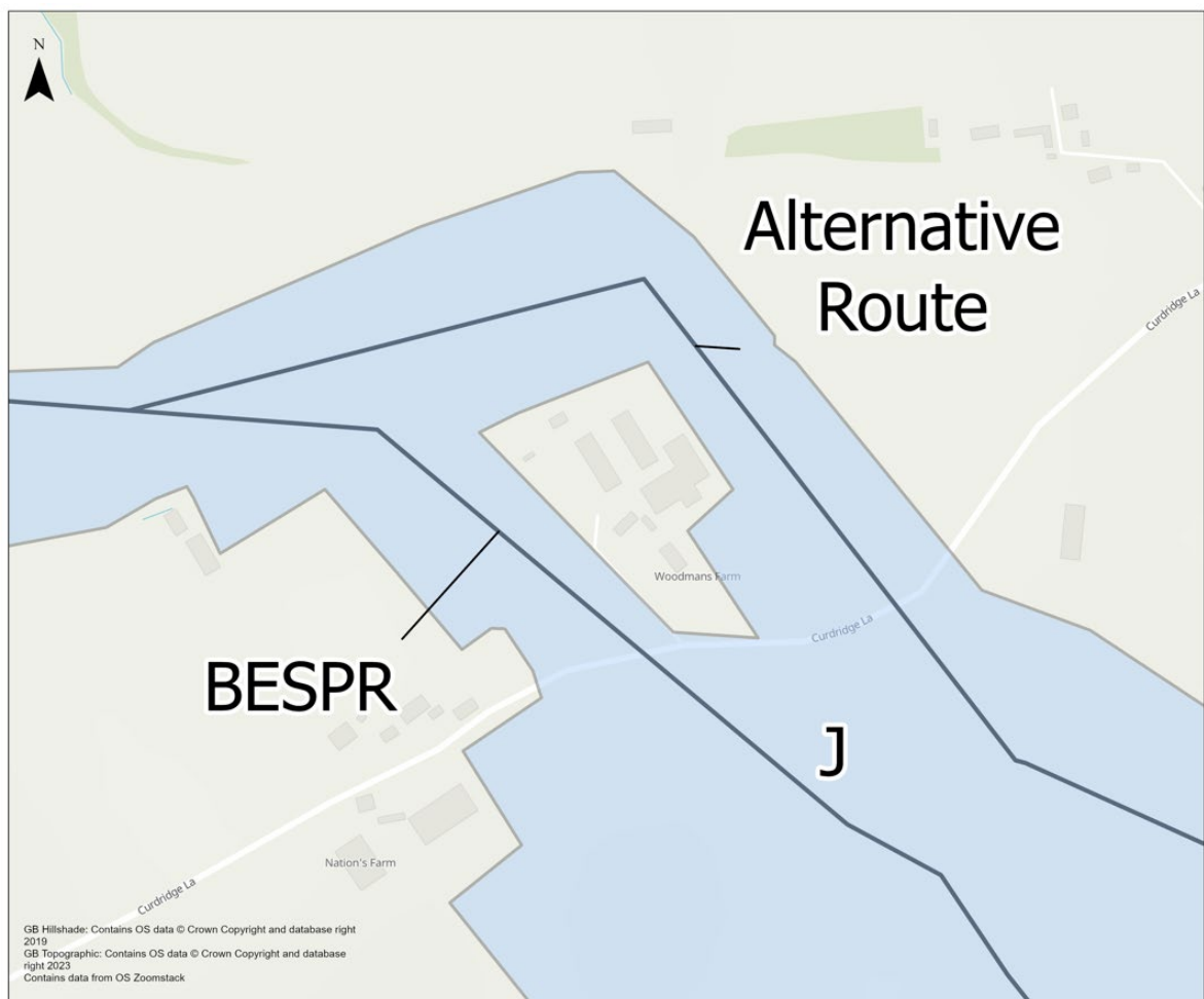
Figure 33 - Section J pipeline options at Woodmans Farm
